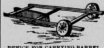
DEVICE FOR CARRYING BARREL. Round down the ends of the three by four inch piece, making about seven inches of each end into a spindle two and one-half inches in diameter.
