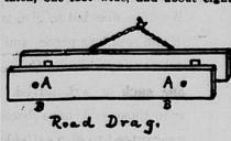
feet long. The sketch shows its construction. Use short sections of oak to hold the two planks about 28 inches apart. Shoe the lower front edges.
